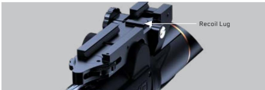
With the clamping nuts loose, push the scope forward until there is firm metal to metal contact on the recoil lug. Tighten both bolts to 40 to 70 in-lbs.
