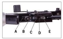
**C)** Adjusts the 1st stage travel - this screw contacts the bottom sear, adjusting clock-wise decreases travel, counter clockwise will increase the travel.
