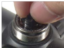
J-5 Apply gentle force on the plastic tab and dial the knob.
