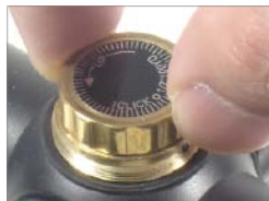
J-4 Apply gentle force on the rim and dial the knob.
