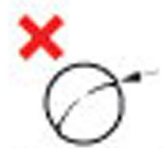
BB with mold line will jam
